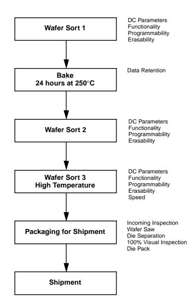
Figure 1. AMD KGD Product Test Flow
